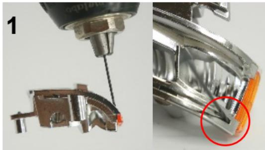
direction. The glued-in orange disk may be slightly scratched when drilling.
